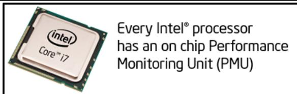
Every Intel® processor has an on chip Performance Monitoring Unit (PMU)
