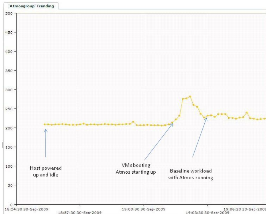
Figure 8. Virtual Machine System Initialization.
