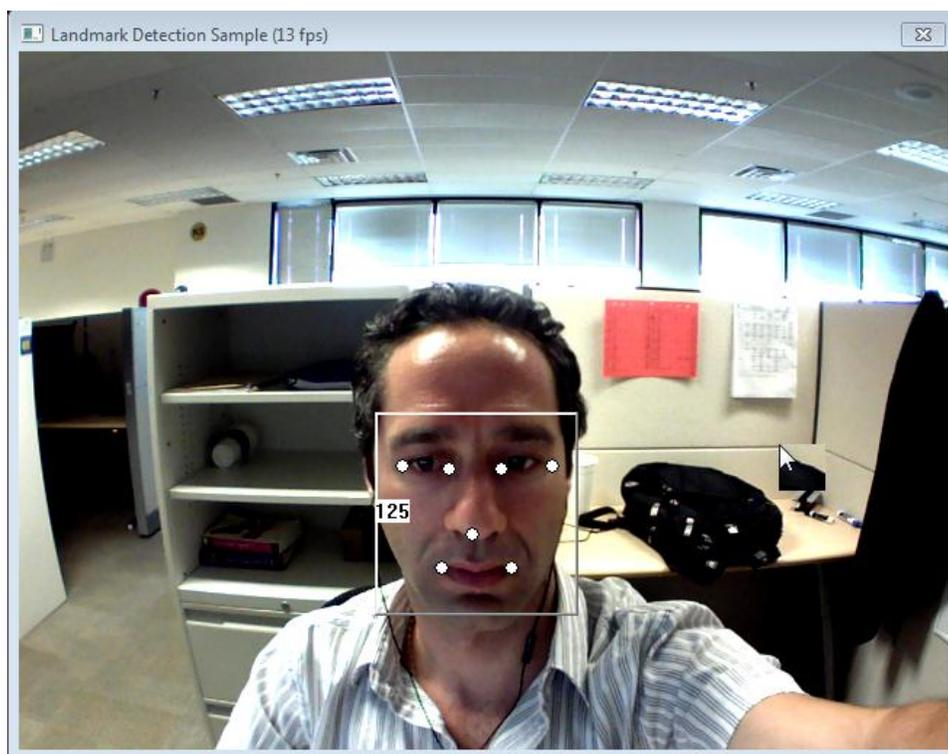
**Figure 2: Face landmark detection, 7 point landmarks.**
