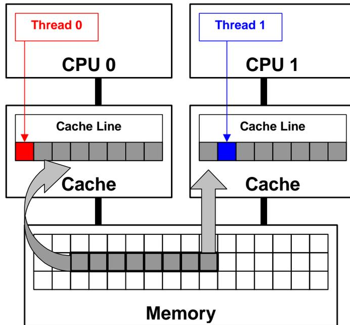
**Figure 1.** False sharing occurs when threads on different processors modify variables that reside on the same cache line. This invalidates the cache line and forces a memory update to maintain cache coherency.
