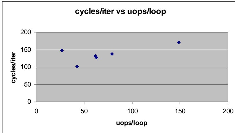
shows a very clear minimum when the number of uops in the inner loop is slightly larger than the RS, meaning that two iterations of the dependent chains of FP operations could be interleaved by the RS.
