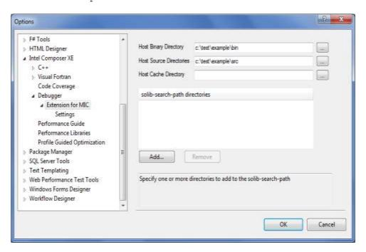
For "Host Binary Directory" specify the directory containing (a copy of) the binary that is to be debugged on the coprocessor. The root directory for finding the sources can be specified by "Host Source Directory". Optionally search paths to shared libraries for the coprocessor application can be added in the "solib-search-path directories" text field. The semantic is the same as for GNU\* GDB.
