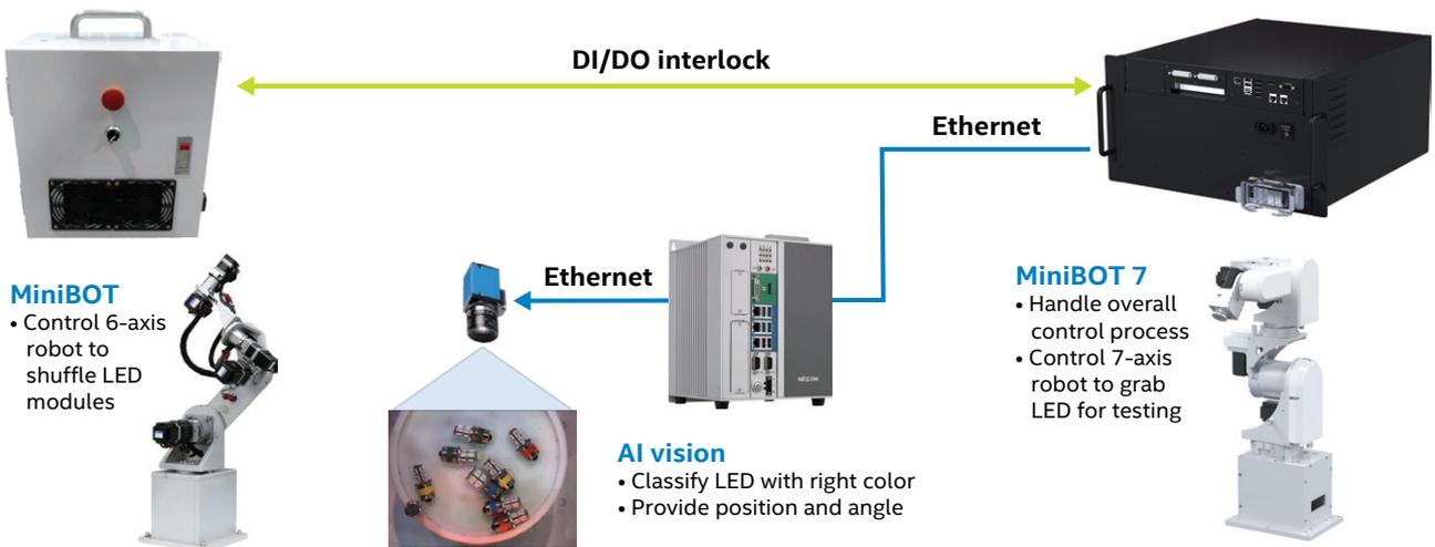
The robotics solution from NexCOBOT integrates machine vision and AI powered by high-performance Intel® architecture
