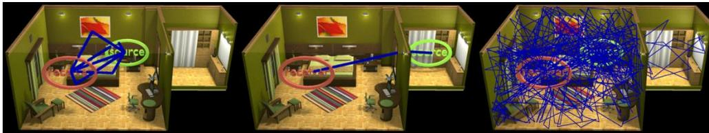
Figure 1: Example scene showing (left) specular, (middle) diffraction, and (right) diffuse propagation paths.
